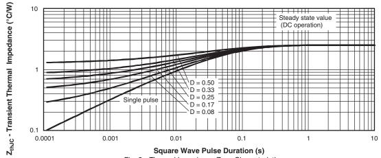
Fig. 8 - Thermal Impedance ZthJC Characteristics
