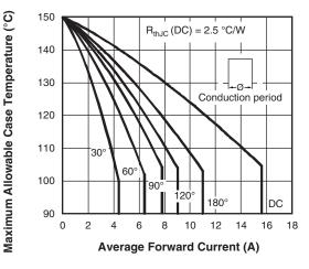
Fig. 2 - Current Rating Characteristics
