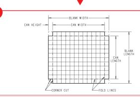
Use this diagram as a guide when cutting your etched Shield Can Sheets.
