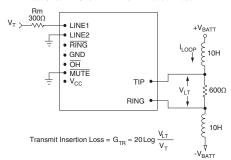
Test Circuit 2: CYG2111 Receive Insertion Loss
