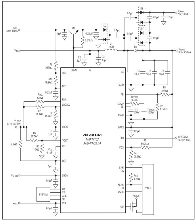
Figure 1. MAX17103 Typical Operating Circuit
