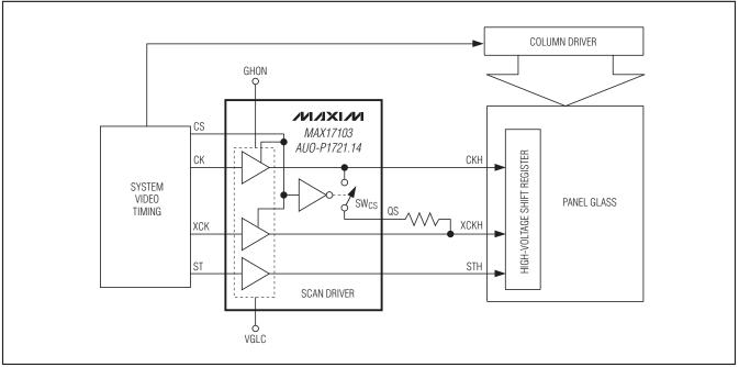
Figure 4. Scan Driver System Diagram
