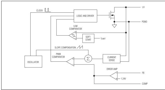
Figure 3. Step-Up Regulator Block Diagram
