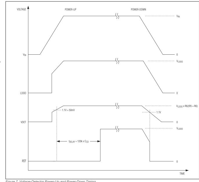
Figure 7. Voltage-Detector Power-Up and Power-Down Timing
