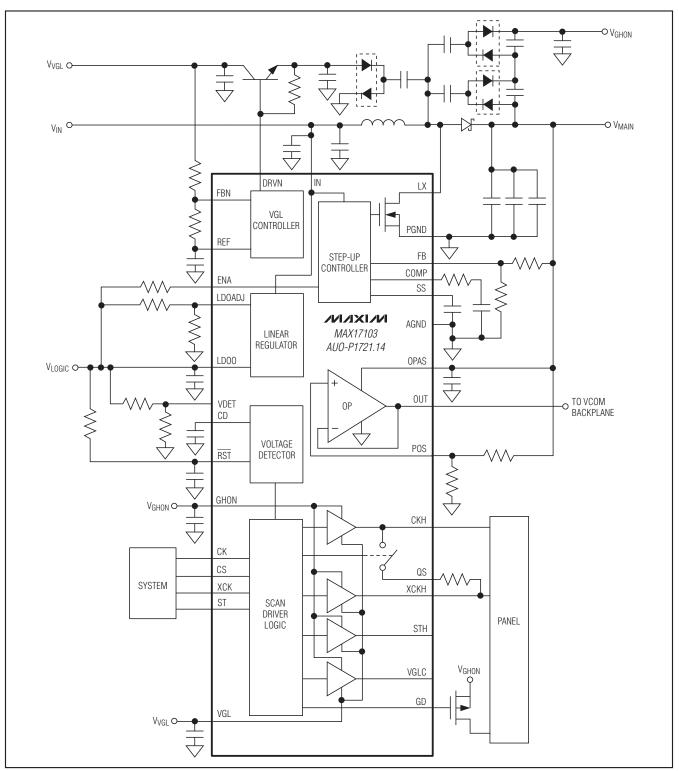
Figure 2. MAX17103 Functional Diagram
