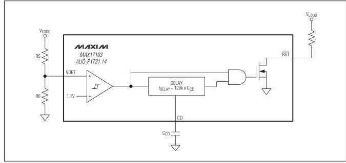
Figure 6. Typical Voltage-Detector Configuration
