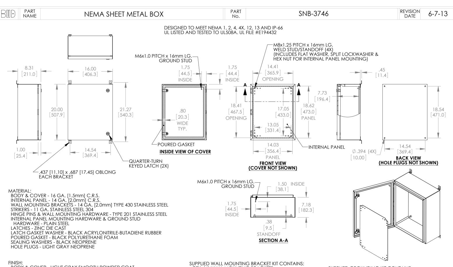
BODY & COVER - LIGHT GRAY SMOOTH POWDER COAT INTERNAL PANEL, INTERNAL PANEL MOUNTING HARDWARE & GROUND STUD HARDWARE - CLEAR ZINC PLATED WALL MOUNTING BRACKETS, STRIKERS & HINGE PINS - NATURAL LATCHES - CHROME PLATED
