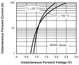
Fig. 7 - Forward Voltage Drop Characteristics
