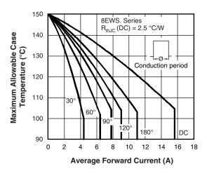
Fig. 2 - Current Rating Characteristics
