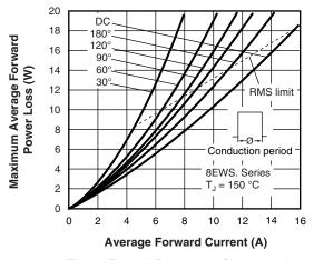
Fig. 4 - Forward Power Loss Characteristics
