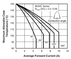
Fig. 1 - Current Rating Characteristics
