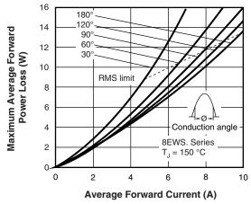
Fig. 3 - Forward Power Loss Characteristics
