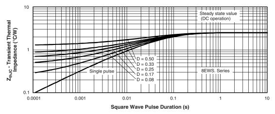
Fig. 8 - Thermal Impedance  $Z_{thJC}$  Characteristics
