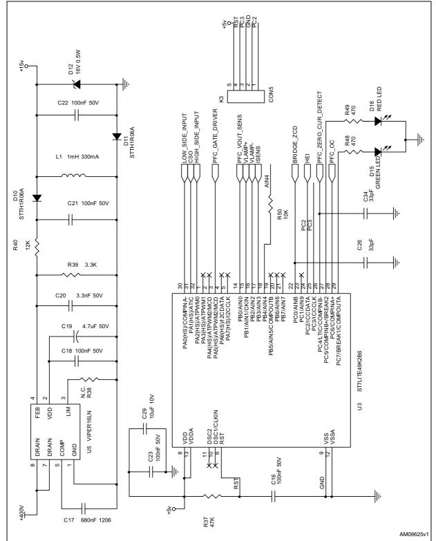
Figure 3. Auxiliary power supply schematic and microcontroller pin functions
