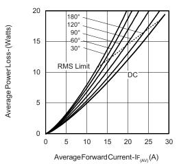
Fig. 6 - Forward Power Loss Characteristics
