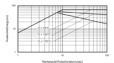
Fig. 9 - Reverse Bias Safe Operating Area (Avalanche Energy vs. Rectangular Pulse Duration)
