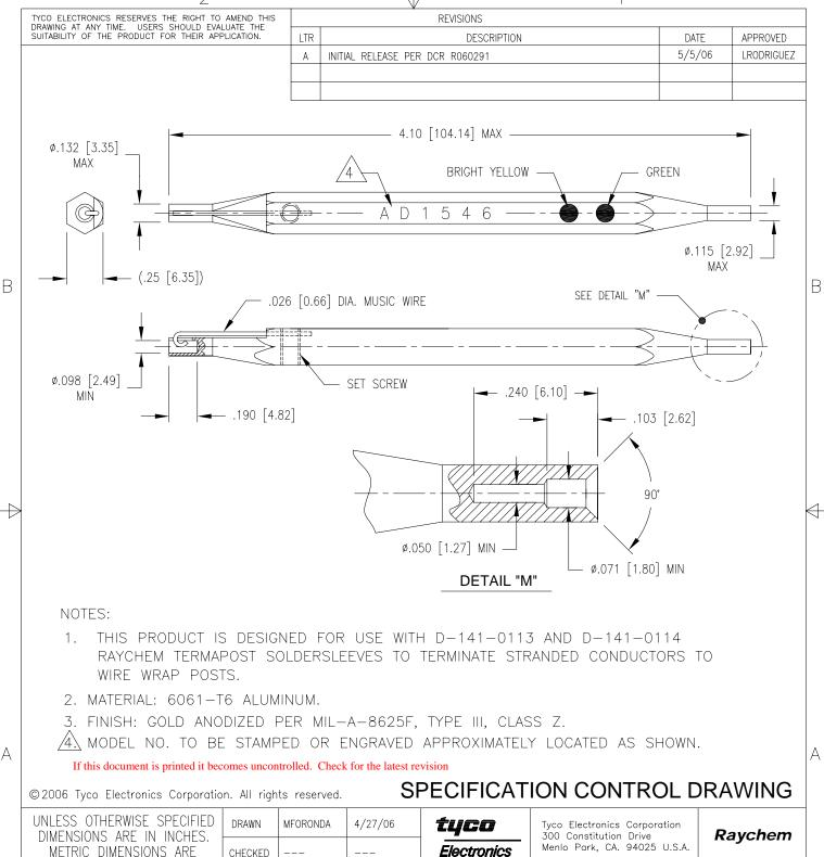
IN BRACKETS. TITI F **APPROVED** DECIMALS INSTALLATION TOOL FOR  $.XXX \pm 0.005$  [ 0.13 mm] REVISED D-141-0113 AND D-141-01140.25 mml ± 0.01 CAD NAME: SOLDERSLEEVES R060291.dwg 0.50 mm] . X  $\pm 0.1$ CODE IDENT. NO. DWG. NO. SIZE **ANGLES** AD-1546 THIRD ANGLE 06090 Χ. ± 0.5 DEG **PROJECTION** DO NOT SCALE THIS DRAWING SHEET 1 OF
