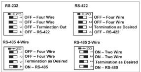
Figure 5. Serial Settings - DIP Switch Configuration
