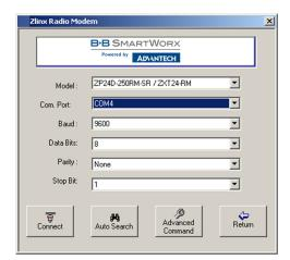
Figure 2. Communication Parameters Screen
